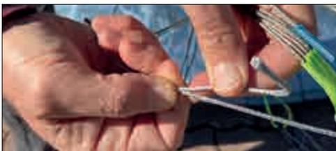
4- To adjust the lengths of the lines, use the sliding splices, a small end of the line that comes out in the extension of the connection to be adjusted, and pull it to adjust its length.
