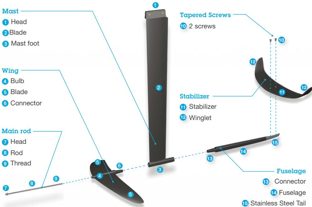
The front and rear wings work as lifting devices, which means they can create a lifting force from the flow of water that travels across them at speed. This is the reason why they are built with a specific sectional profile:
