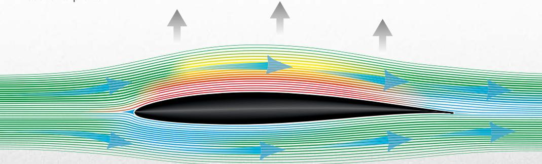
The shape of the wings' profile shall not be modified, filled and sanded. Doing so would alter the balance and prevent the correct operation of the kitefoil.
